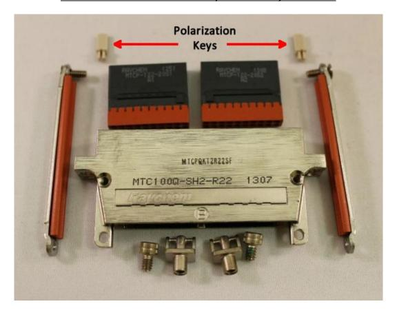
As you can see in the picture above, we purchase and ship the connector without the last two digits specified for one of the 16 possible polarizations. e.g. MTCPQKT2R22SFAB
