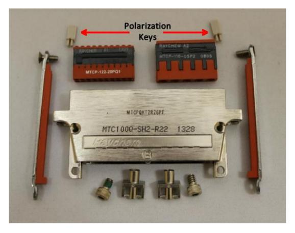
As you can see in the picture above, we purchase and ship the connector without the last two digits specified for one of the 16 possible polarizations. e.g. MTCPQKT2R26PFAB
